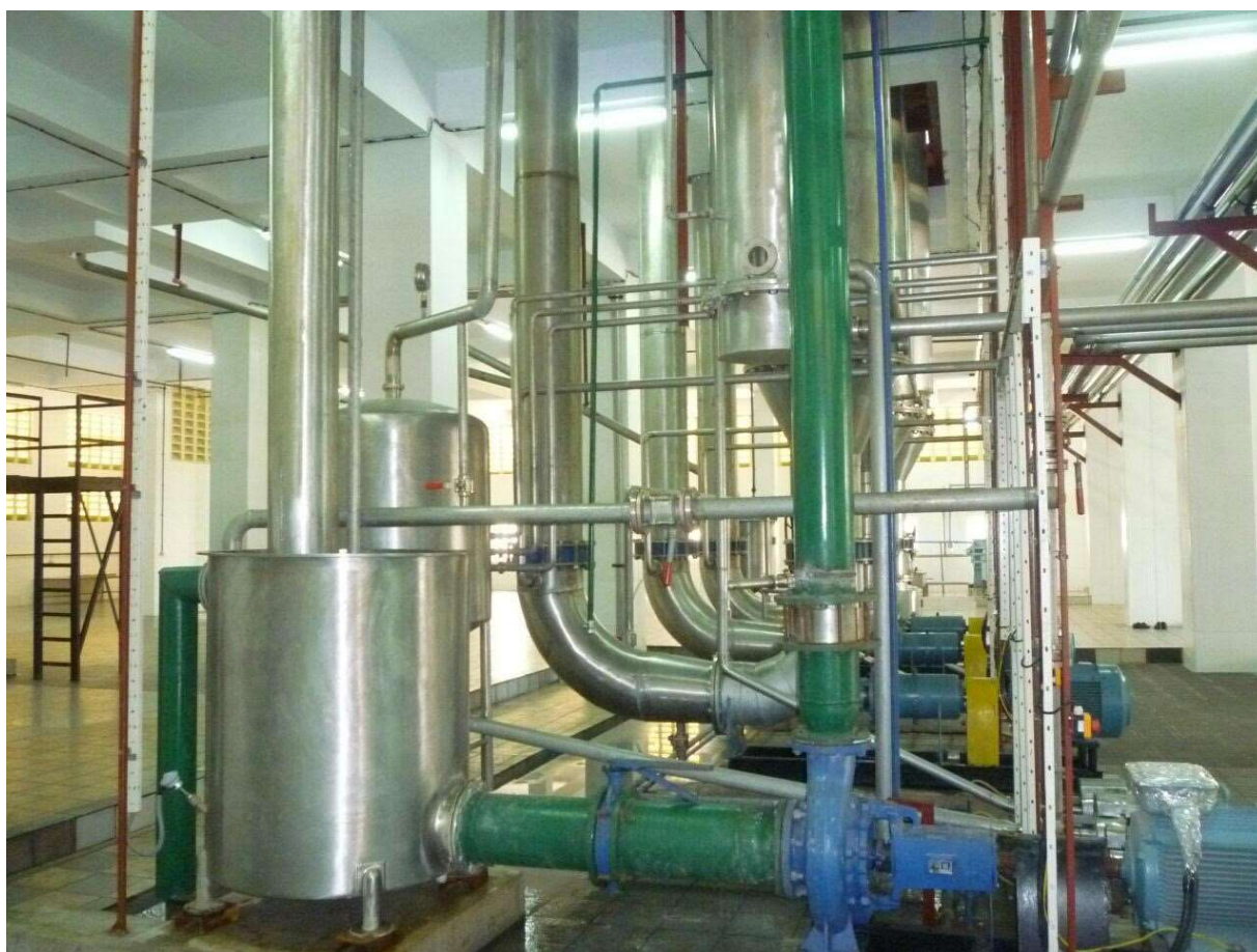
Picture 6 Kensalt 3-effect, 5 tph vacuum salt refining plant in Mombasa
